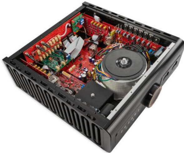
A large toroidal transformer feeds the preamp section at the rear and power amp circuitry that's bolted to the left and right heatsinks
